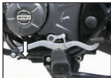
Gear shifting pattern - All Up- Discover 110
