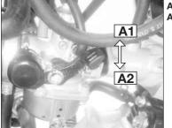
A1 : ON A2 : OFF  When the engine is warmed up enough to idle without using choke, return the choke to OFF position.
