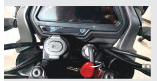
Mobile charging socket is provided near Ignition switch as an OE fitment.
