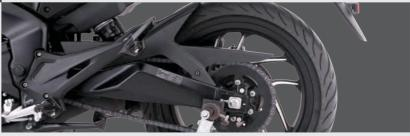
Ensure application of 9 to 11 Kgf.m torque to rear axle nut.
