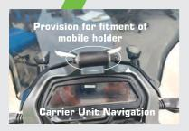
Provision for fitment of mobile holder a carrier unit navigation is provided above speedometer as an OE fitment.
