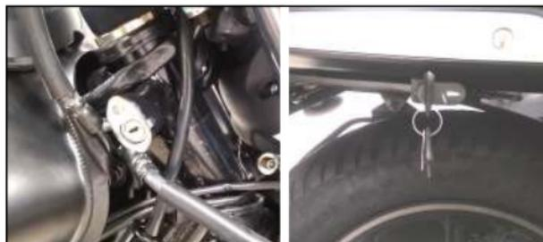
**Ignition Lock :** It is located at right side of the frame below 'Fuel Tank'. It has 2 positions. The key can be removed from switch only in 'OFF' position.
