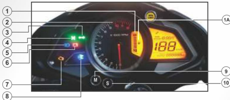
**1. Fuel Level Indicator:** It shows fuel level in fuel tank.
