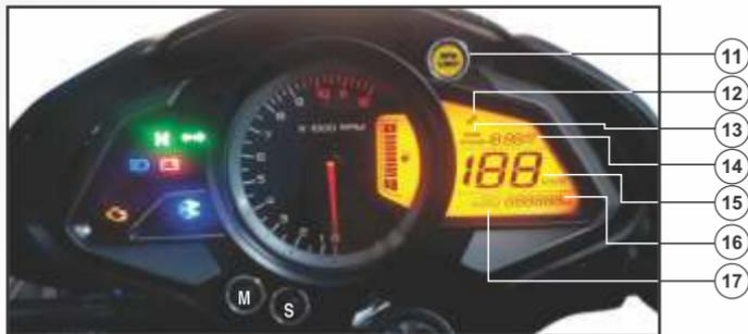
**11. Engine Rev Indicator:** It blinks when engine RPM is between 9500 to 10000 RPM. Continuously ON at RPM more than 10000.
